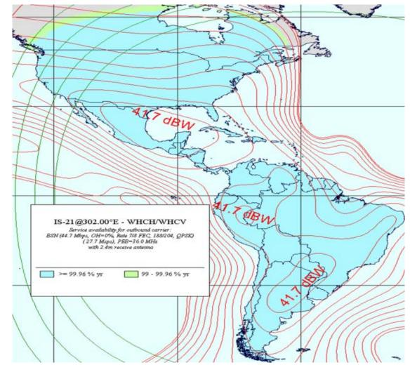
IS21 C-Band Coverage Estimate for 2.4 Receive Antenna
