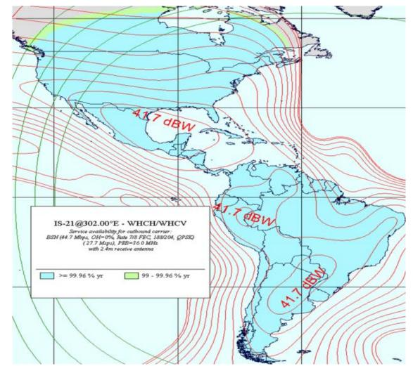
IS21 C-Band Coverage Estimate for 1.8 Receive Antenna
