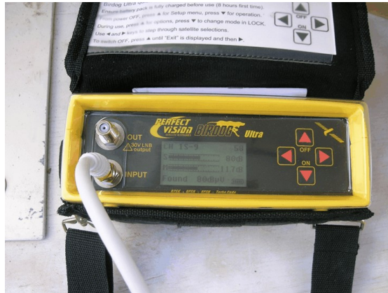
Photo of the Birdog, which is a satellite finder and signal meter we used as part of a test installation. While not strictly necessary for deployments, it is certainly a lot handier than attempting to find a signal with the dish attached to your DVB-S receiver using the receiver software on your computer to test for a lock.
