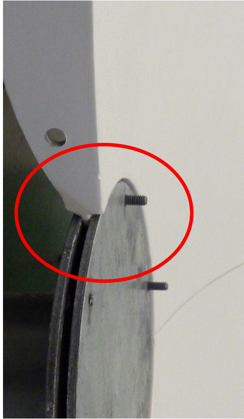
Photo of center hub and center plate attached to reflector with one petal removed. The center hub is attached to the center plate with bolts. The two, when bolted together 'pinch' the lip of the petals.
