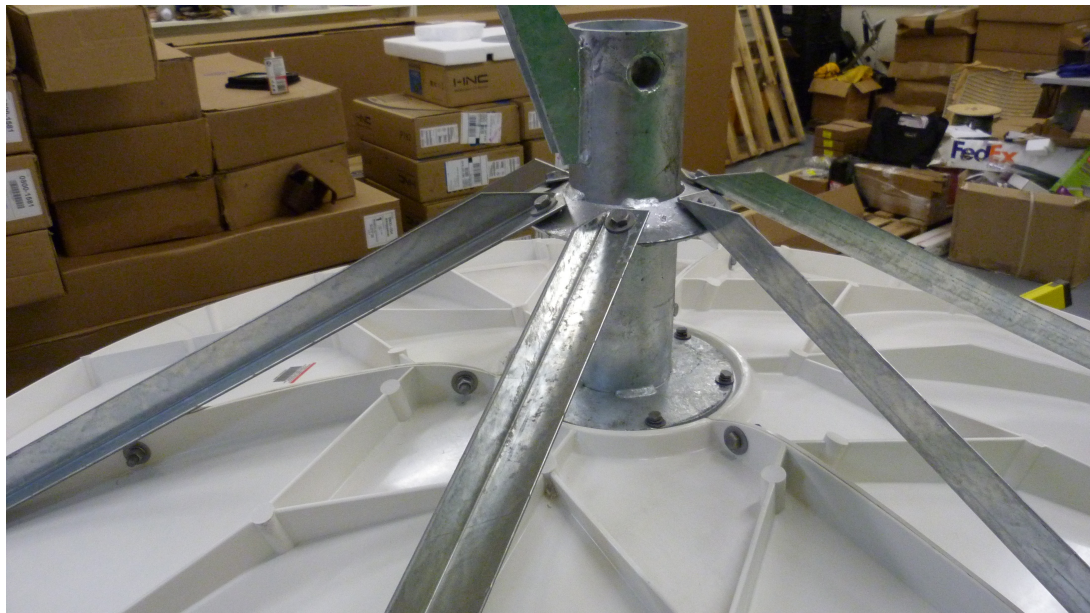
Photo of center hub with angle braces attached to the back of the reflector dish.
