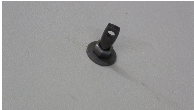
Photo of feed support bolt. Note that attachment hole is on the face side of the reflector.
