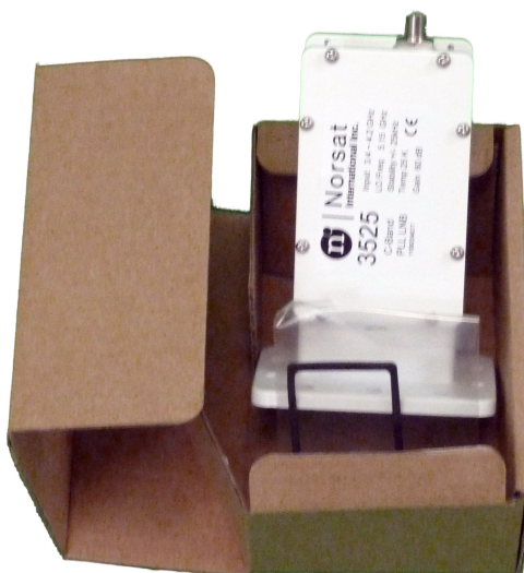
Photo of Norsat LNB just opened from box. With the LNB is a gasket to help with seal to feed horn.
